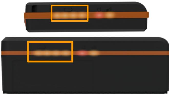
While charging, the battery LEDs display the charge of the device like a power bank:
